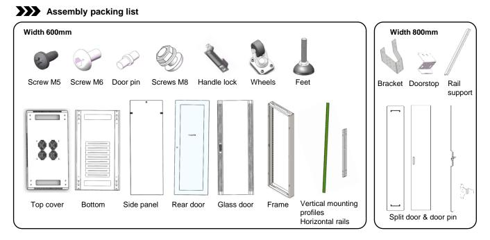
Step 1: Fix the top cover and bottom on frames with M8 screw; Fix the wheels on bottom panel.
